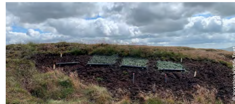
Figure 24: Enabling the revegetation of bare peat using hydroseeding. All the different Peat Fix treatments tested enable vegetation establishment and significantly reduce peat erosion.
