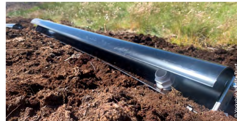
Figure 23: Collecting the peat eroded from test plots. Innovative new sediment traps were designed to collect sediment falling to the bottom of slopes on the flanks of peat hags.
